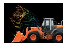
With the new parallel/tandem circuits, the lift arm and bucket can be operated at the same time, unlike conventional machines. This can remarkably increase digging and loading efficiency for higher
