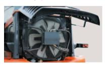
Fan speed can be adjusted depending on fluid temperature to effectively cool down coolant, hydraulic oil, transmission oil and torque converter oil. The result is extended component service life and reduction in fuel consumption. The fan is also separate from the engine for easy servicing.
