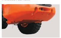
The large counterweight is arranged to protect the fuel tank from collisions with obstacles during operation.
