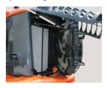
The rotation of the hydraulically operated cooling fan with heat-sensing system can be reversed for easy removal of dirt from the radiator. The fan itself can swing open for easy cleaning.
