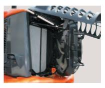
The radiator and oil cooler are made of aluminum instead of conventional steel or copper for corrosion protection.
