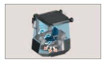
The bi-level air conditioner allows air conditioning at foot space and overhead simultaneously. Airflow volume and direction can automatically be adjusted according to the temperature setting. The pressurized cab shuts out dust and debris even in dusty environment.
