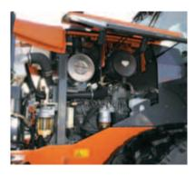
Dual fuel filters with sedimentary function and engine oil filter are strategically located for the convenient daily inspection and servicing from the ground.
