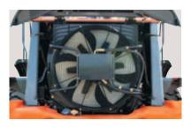
The cooling fan is enclosed by a full guard (metal net) to protect service technicians from injury during servicing and maintenance.
